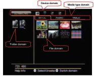
[Tips]: In photo full-screen play, you may press the FUNC button to eject the photo display mode window; with the ♠ and ♥ buttons, you can choose different photo display mode, and press the OK key to confirm.
